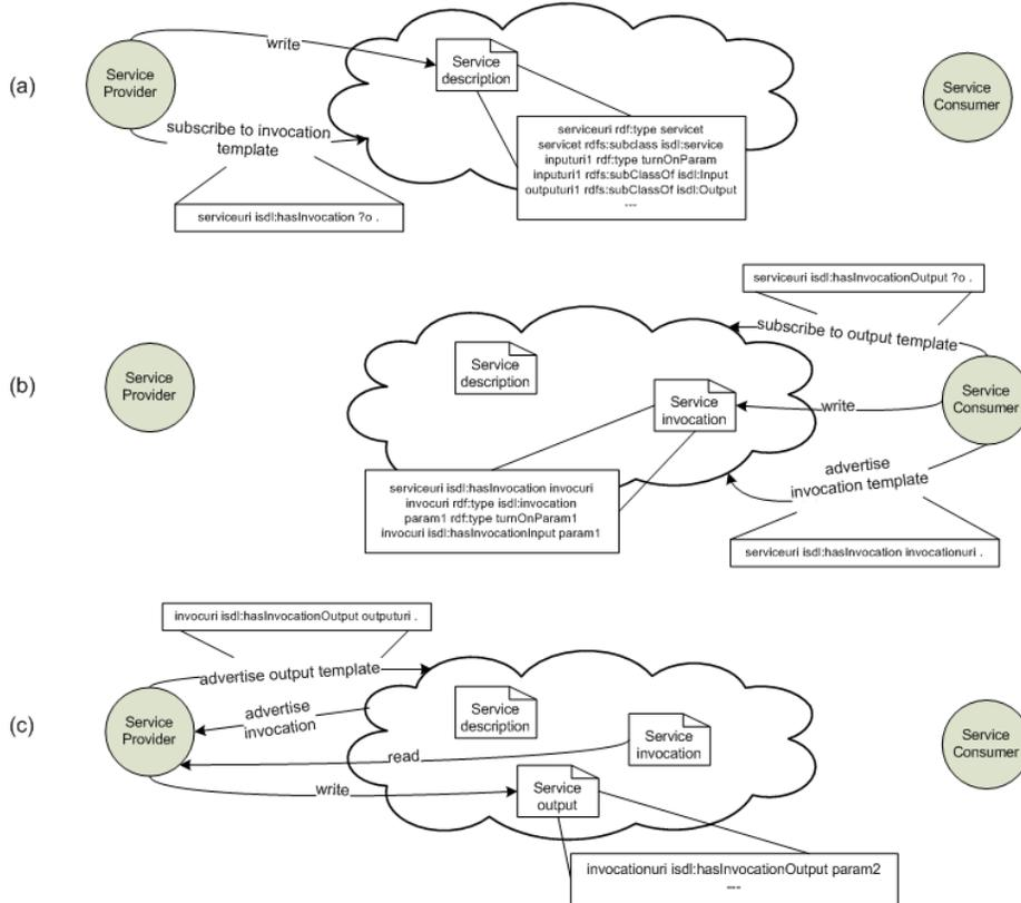
**Fig. 1.** Services over tsc++: a) registration, b) invocation from the consumer point of view and c) invocation from the service provider point of view.
